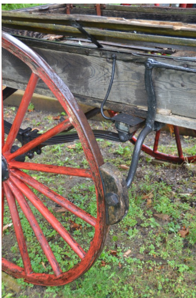
The break lever, above, to activate the breaks on both rear wheels, left. Note the leaf springs and gracefully curved iron brace supporting the sidewall. The side rails, right, are removable, slotting into brackets on the sidewalls.
