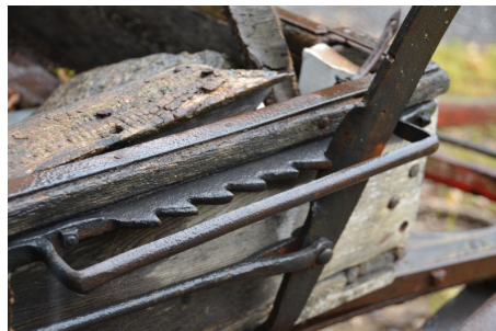
The break lever, above, to activate the breaks on both rear wheels, left. Note the leaf springs and gracefully curved iron brace supporting the sidewall. The side rails, right, are removable, slotting into brackets on the sidewalls.
