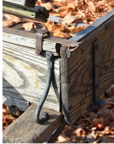
The tailgate can be lowered by operating the sprung thumb-pry latches on either side of the wagon. Note again the curved sidewall brace. The brackets on the inside of the tailgate allow end rails to be installed.
