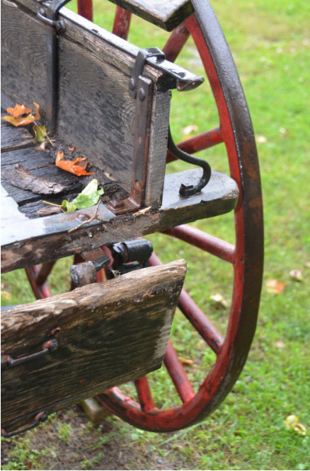
The tailgate can be lowered by operating the sprung thumb-pry latches on either side of the wagon. Note again the curved sidewall brace. The brackets on the inside of the tailgate allow end rails to be installed.
