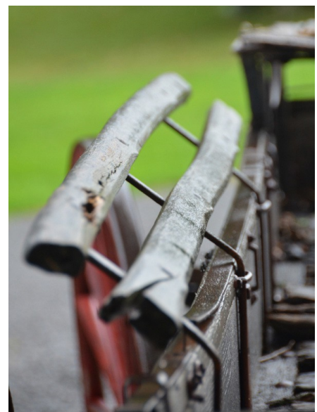
The break lever, above, to activate the breaks on both rear wheels, left. Note the leaf springs and gracefully curved iron brace supporting the sidewall. The side rails, right, are removable, slotting into brackets on the sidewalls.
